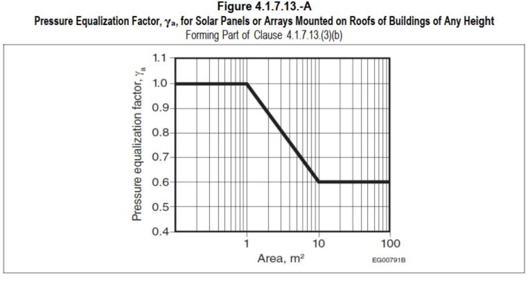
$p = I_W q C_e C_t C_g C_p E \gamma_a$
